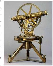
In the most precise long-distance work, signaling lamps or heliographs reflecting the Sun are used as targets for the theodolite. For less demanding work and work over shorter distances, smaller theodolites with simpler reading systems can be used; targets are commonly striped poles or ranging rods held vertical by an assistant.
