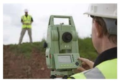
eliminates the need for an assistant staff member as the operator holds the reflector and controls the total station from the observed point.
