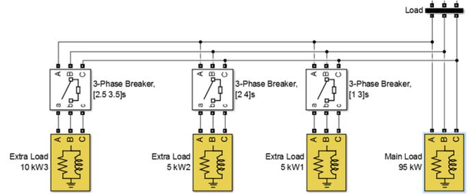
Fig.15. Load Profile modeled in Simulink/MATLAB
