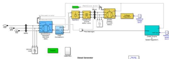
Fig.6. Diesel Generator system Model in Simulink/MATLAB [5]
