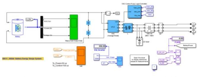
Fig.7. Battery Energy Storage system Model in Simulink/MATLAB [5]
