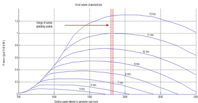
Fig.3. Profile of wind power with respect to the wind speed [5]
