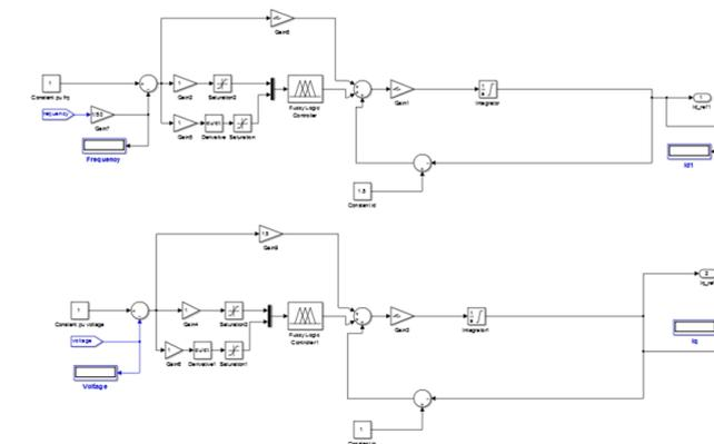
Fig.10. Id and Iq -Fuzzy Logic Controller of VSC in Battery System Model in Simulink/MATLAB
