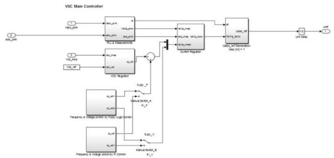
Fig.8. SVC (PI and Fuzzy Logic) Controller of BESS System Model in Simulink/MATLAB
