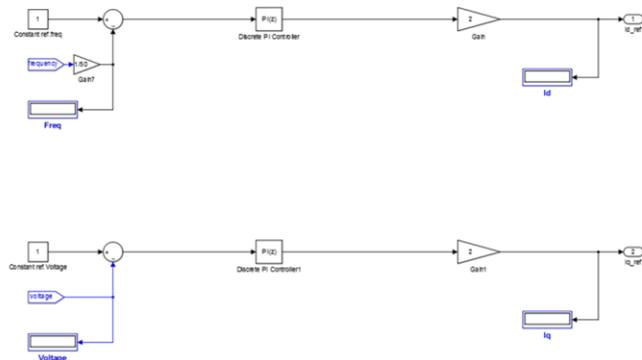
Fig.9. Id and Iq -PI Controller of VSC in Battery System Model in Simulink/MATLAB
