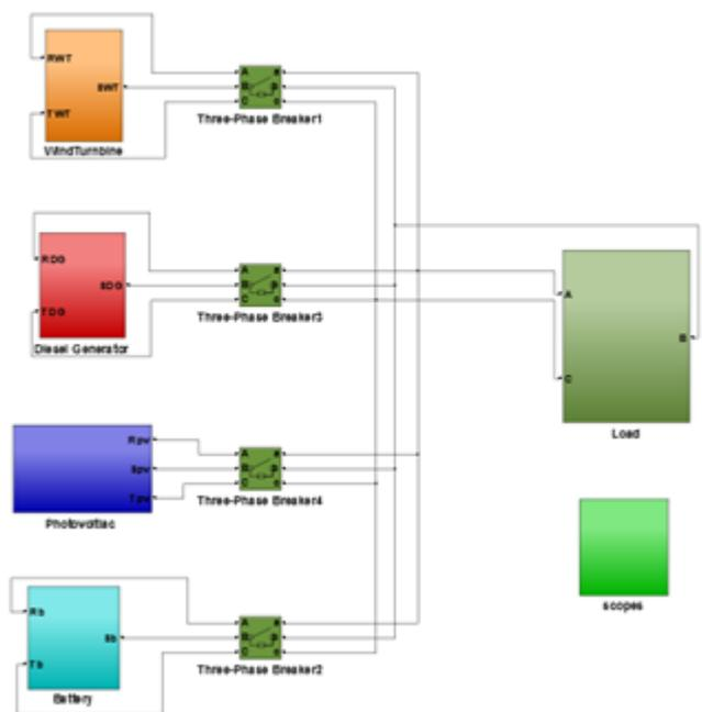
Fig. 1. Standalone Micro Grid Hybrid system modeled in Simulink/MATLAB
