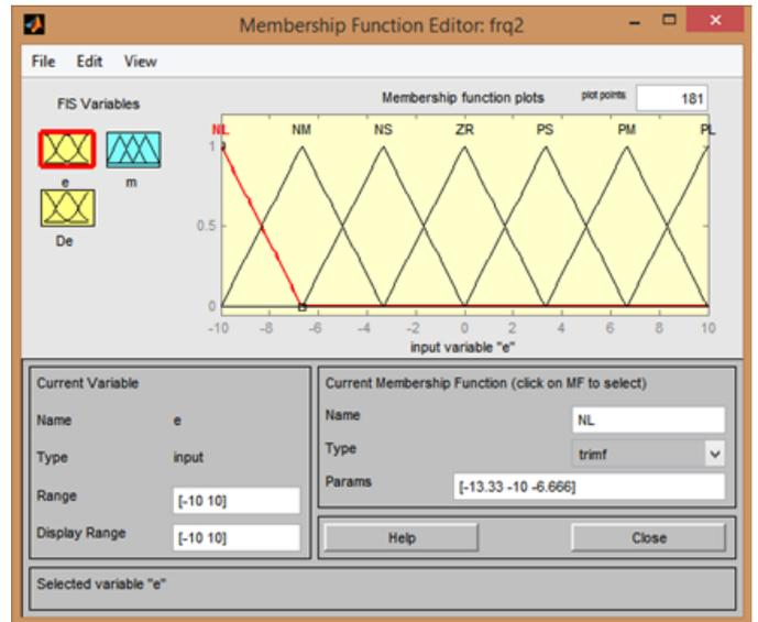
Fig.11. Membership Function for input and output of fuzzy logic system
