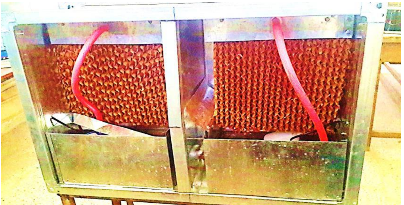
Figure (2) direct evaporative cooling after completed
