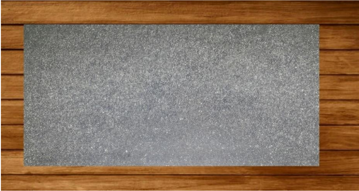
Figure (4) desiccant material coated on both sides of metal element
