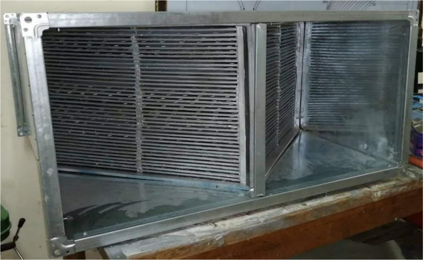
Figure (7) Manufactured heat exchanger after installed in the duct
