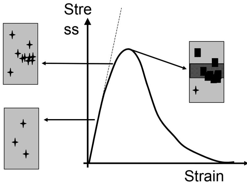
FIGURE 3 Strain softening aggregate and rock.
