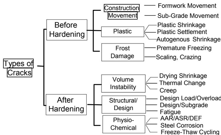
**FIGURE 1 Common causes for cracking in concrete dtructures.**
