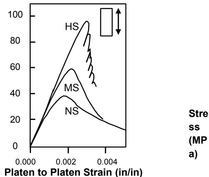
FIGURE 5 Influence of strength on the stress-strain response (1 MPa = 145 psi). crack. Fatigue causes a crack to propagate through the matrix (typically starting along the interfacial zone between an aggregate and the paste). As cyclic loading proceeds, stresses are redistributed and the macro-crack width decreases but never closes completely.
