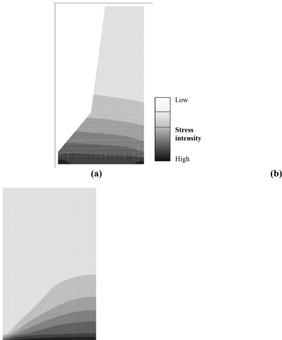
FIGURE 10 Longitudinal stress distribution along an RC barrier under uniform shrinkage: (a) height, and (b) length.
