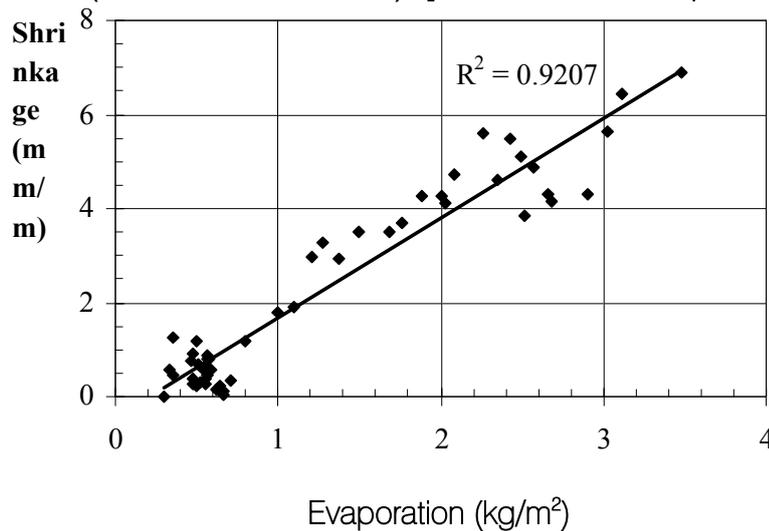
FIGURE 7 Early age shrinkage dependence on evaporation prior to setting for normal strength concretes (Holt and Leivo, 2000). [1 mm/m = 0.001 in./in., 1 kg/m<sup>2</sup> = 0.2 lb/ft<sup>2</sup>.]
