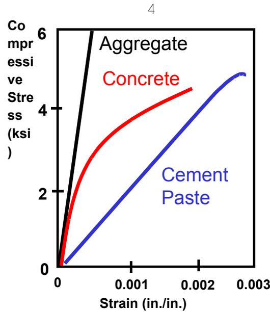
FIGURE 2 Stress strain response of behavior of concrete (1 ksi = 6.89 MPa).
