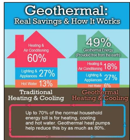
escape the effects of freezing temperatures. The ground there stays close to 60 degrees Fahrenheit (15.5 degrees Celsius), making it a warm source of energy in winter and a cool source of energy in summer (*greensolarcafe.com/solar-wind-hydro-renewable-energy/geothermal-heating-and-cooling/*)
