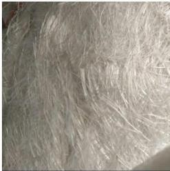
Polyester fibers are used in fiber-reinforced concrete for industrial and warehouse floors, pavements and overlays and precast products. Polyester micro- and macro-fibers are used in concrete to provide superior resistance to the formation of plastic shrinkage cracks versus welded wire fabric and to enhance toughness and the ability to deliver structural capacity.
