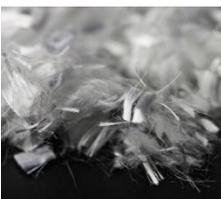
Micro-synthetic has a diameter that is less than 0.3 mm. Provide superior resistance to the formation of plastic shrinkage cracks (cracking that occur in
