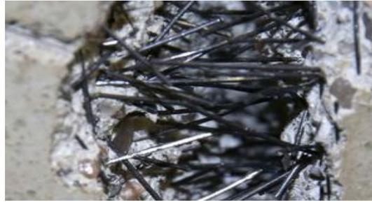
$\gamma^{\text{nd}}$  – Fiber makes the concrete more impermeable
