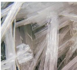
Polypropylene fiber which is classified as number 0-PP (plastic polymer). Transformed from propylene, it has similar properties as polyethylene but it is harder and more heat resistant, used in a variety of applications.
