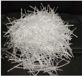
Polymer fiber bars (PFB) is made from Ethylene and depend on how it polymerizes, it has been widely used in civil engineering and substitutes as steel reinforcement because it has many advantages such as high strength-to-weight ratio, light weight, handling easily and no corrosion. PFB has become an economical and competitive structure material.
