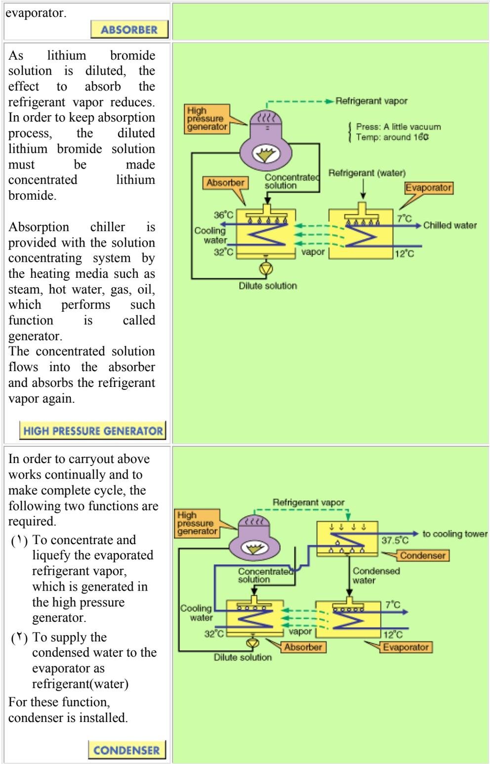
A typical schematic of the absorption refrigeration system is given in the Figure 1.3.
