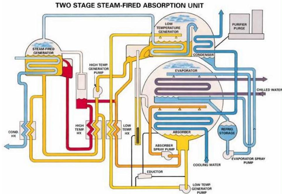
Figure 1.3 Schematic of Absorption Refrigeration System
