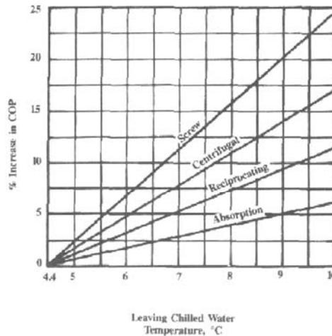
Figure 1.8 Effect Of Evaporator Temperature On Chiller COP
