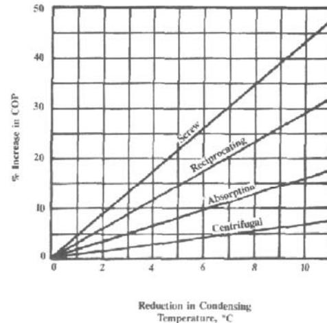
Figure 1.9 Effect Of Condensing Temperature On Chiller COP
