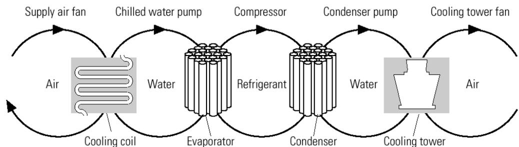
Figure 1.1 Heat Transfer Loops In Refrigeration System
