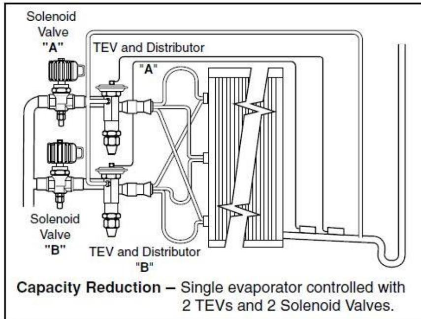
Capacity is accomplished by closing a solenoid valve which deactivates the circuits being fed by the TEV and distributor downstream of the solenoid valve. This method of capacity control, however, requires a degree of care since the heat load on the evaporator circuits will be affected in the manner
