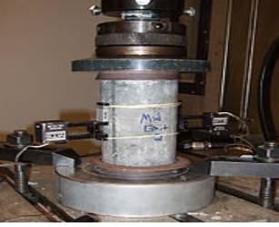
Compression testing of a concrete cylinder.
