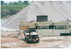
Once processed, the aggregates are handled and stored in a way that minimizes segregation and degradation and prevents contamination. Aggregates strongly influence concrete's freshly mixed and hardened properties, mixture proportions, and economy. Consequently, selection of aggregates is an important process. Although some variation in aggregate properties is expected, characteristics that are considered when selecting aggregate include:
