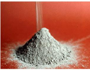
Portland cement, the basic ingredient of concrete, is a closely controlled chemical combination of calcium, silicon, aluminum, iron and small amounts of other ingredients to which gypsum is added in the
