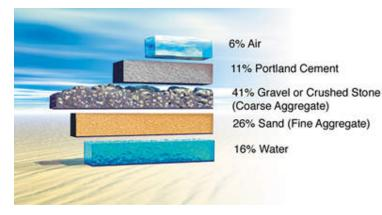
In its simplest form, concrete is a mixture of paste and aggregates. The paste, composed of portland cement and water, coats the surface of the fine and coarse aggregates. Through a chemical reaction called hydration, the paste hardens and gains strength to form the rock-like mass known as concrete.
