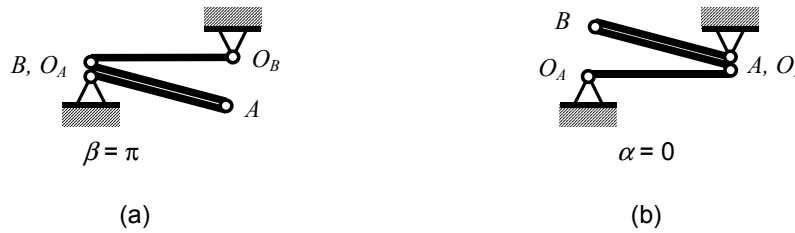
Figure 3.10: Configurations corresponding to the compatibility paths of the square-shaped four-bar mechanism at bifurcation point (\alpha = 0, \beta = \pi) . (a) \beta = \pi and \alpha is varying. (b) \alpha = 0 and \beta is varying.
