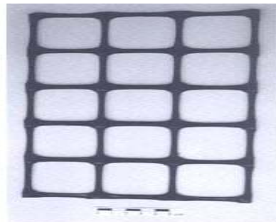
Fig. Uniaxial and Biaxial Geogrids manufactured by the method of extrusion
