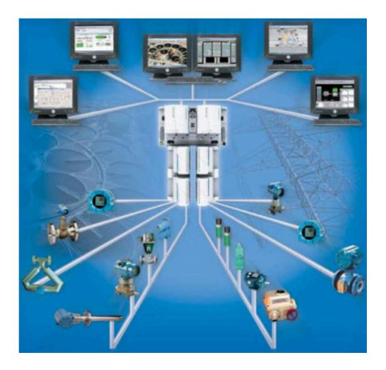
The collected information is further processed, analyzed and produces the output results based on the control logic implemented in the controller. The results or control actions are then carried to the actuator devices via field bus. The DCS configuring, commissioning and control logic implementation are carried at the engineering station as mentioned earlier. The operator able to view and send control actions manually at operation stations
