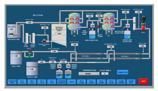
Operating stations can be a single unit or multiple units where a single unit performs functions like parameter value display, trend display, alarming, etc. while multiple units or PCs performs individual functions such as some PCs display parameters, some for trend archives, some for data logging and acquiring, etc
