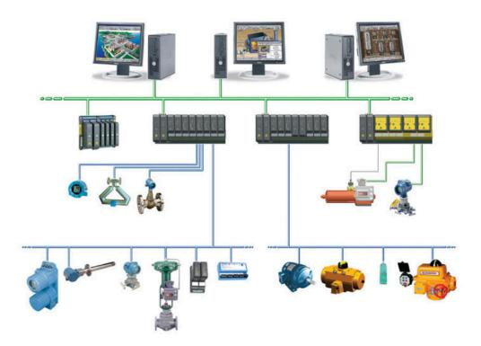
A distributed control system (DCS) is a specially designed automated control system that consists of geographically distributed control elements over the plant or control area.
