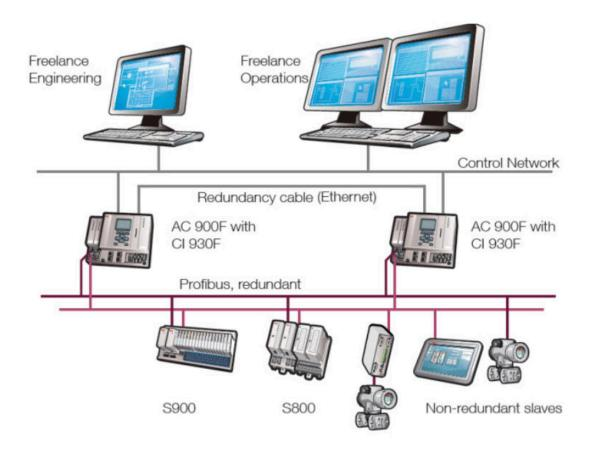
The major advantage of DCS is the redundancy of some or all levels of the control area. Most of the cases critical processes are installed with redundant controllers and redundant communication networks such that problem in main processing line should not affect the monitoring and control functions because of the redundant processing section
