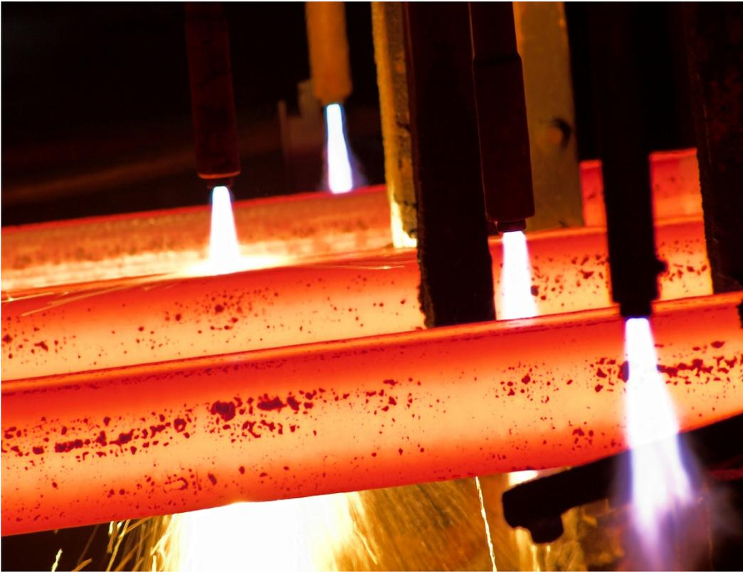
Fig. 7 cutting by gas torches
