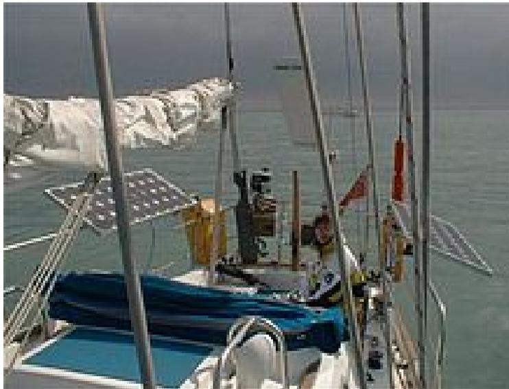
PV used for auxiliary power on a yacht
