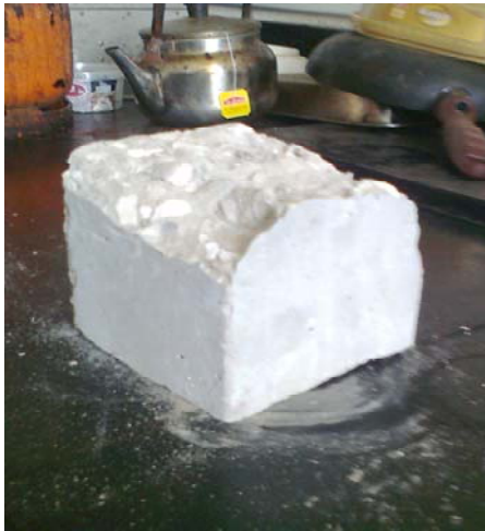
Fig 3.8: Concrete samples containing 100 grams of powdered glass.
