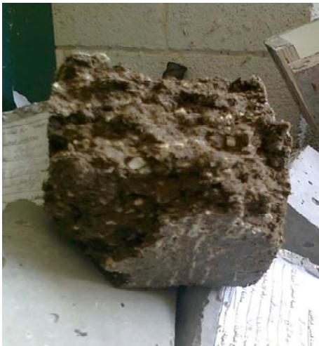
Fig ۳.۴: Concrete sample containing ۱۰۰ grams of rough wood shavings.
