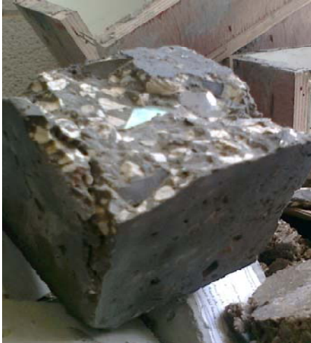
Fig 3.6: Concrete samples containing 4 CD's broken.
