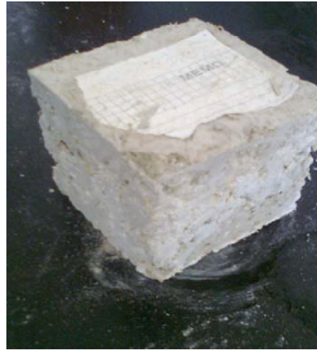
Fig ۳.۵: Concrete sample with added straw (hay ground) ۱۰ grams per cubic.
