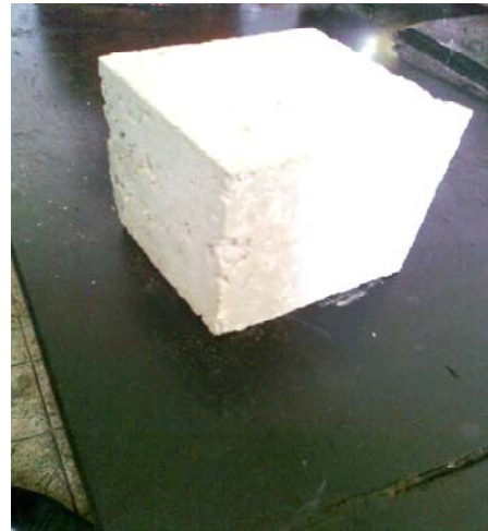
Fig 3.9: Concrete sample containing 2.6 kg cement and 6.0 kg of sand and 12.0 kg aggregate and the strength of concrete is 248kg/cm 2 .
