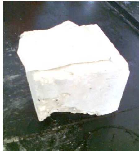
Fig 3.7: Concrete samples containing 70 g of glass and 100 g ash
