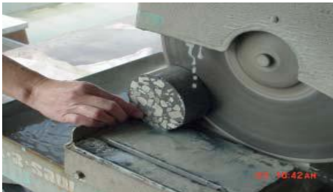
Figure.2 Cutting the 2. Slice for Testing.
