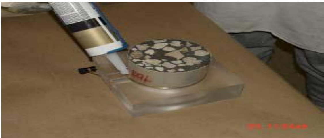
Figure.5 Siliconing Sample into the Test Cell
