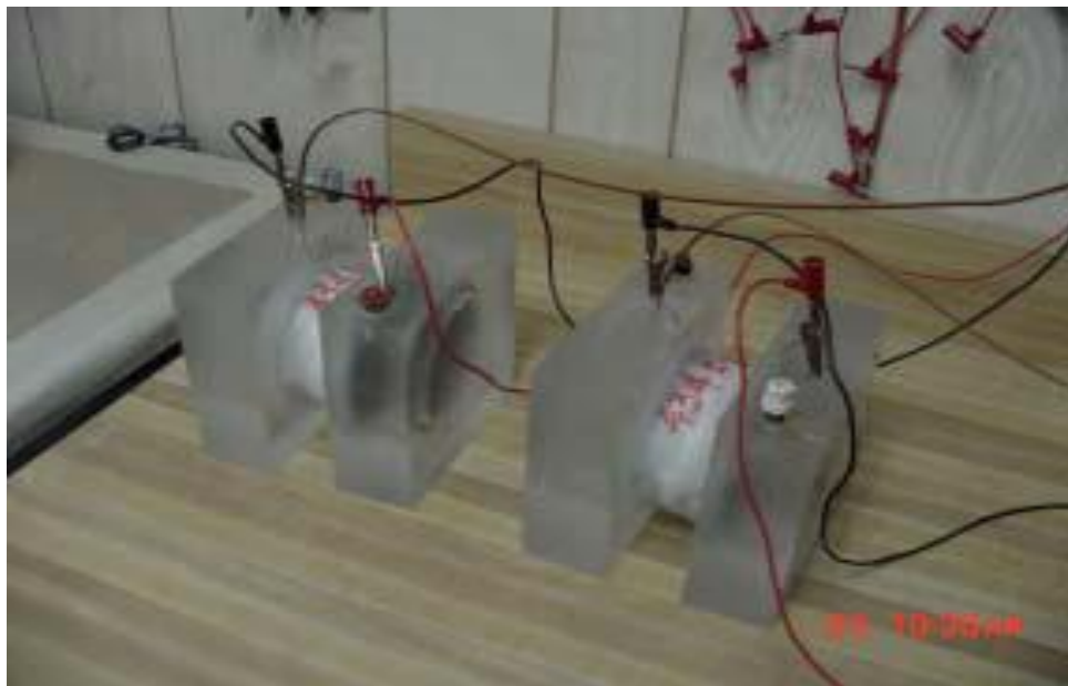
Figure.7 The Complete Testing Configuration (Sample A and B)
