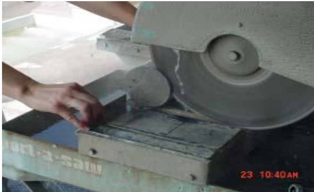
Figure 1. Cutting a \frac{1}{4} . Slice off the Sample to Dress the Troweled Edge.
