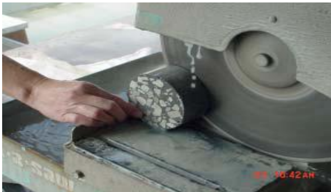
Figure.2 Cutting the 2. Slice for Testing.
