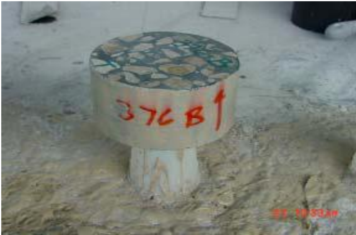
Figure 3 Application of Epoxy around the Samples Circumference
