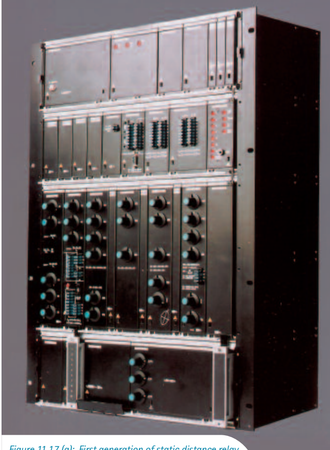
Figure 11.17 (a): First generation of static distance relay
