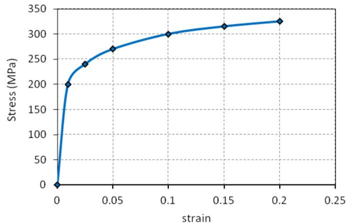
Fig. 3. Engineering stress-strain relationship for steel used in analysis
