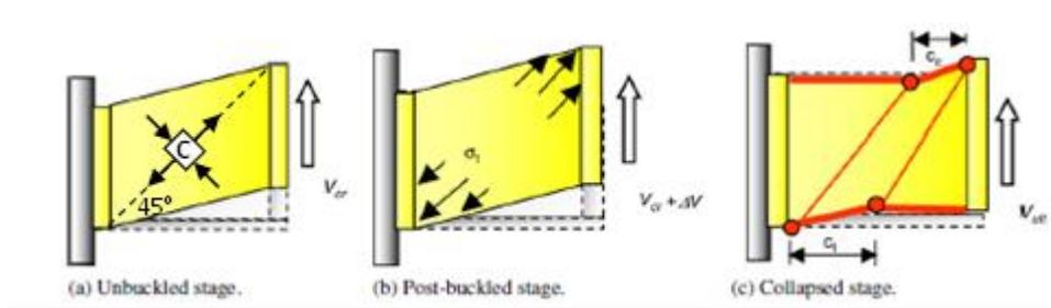
Fig. 1. Web Panel behavior under pure shear
