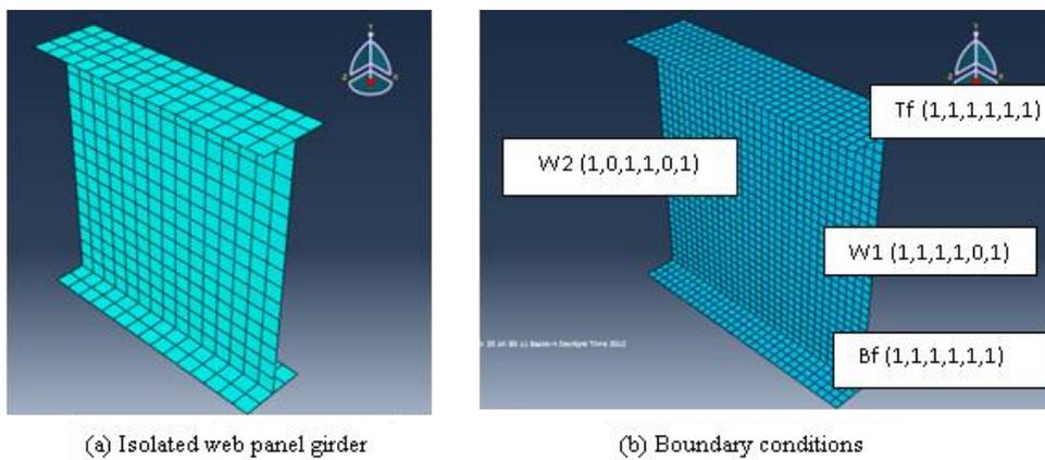
Fig. 2. Web panel girder used in analysis
