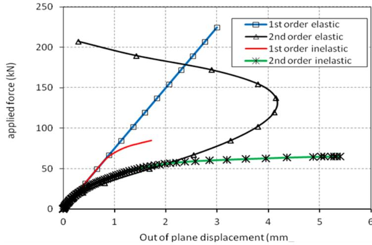
Fig. 6. Web panel girder response for different analysis cases
