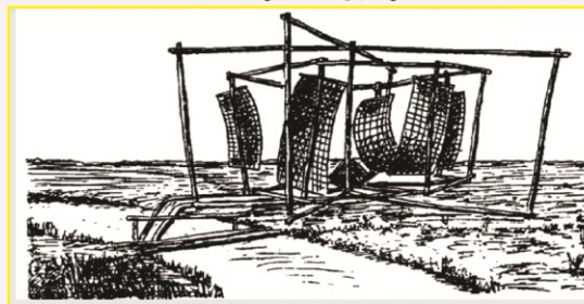
Chinese Windmill (1000 A.D.): independent of wind direction
