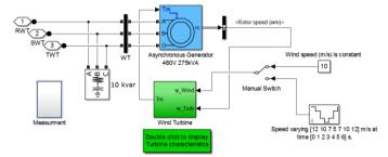
Fig. 2. Wind Turbine Synchronous Generator System Model in Simulink/MATLAB [5]
