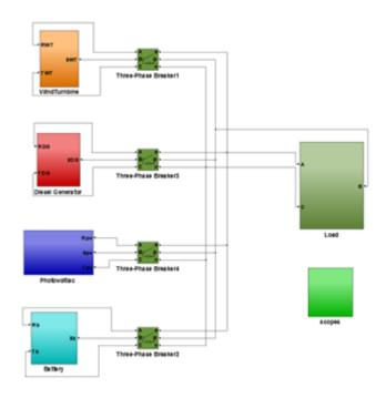
Fig. 1. Standalone Micro Grid Hybrid system modeled in Simulink/MATLAB
