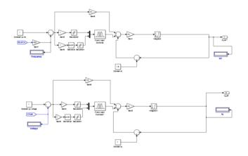
Fig.10. Id and Iq -Fuzzy Logic Controller of VSC in Battery System Model in Simulink/MATLAB
